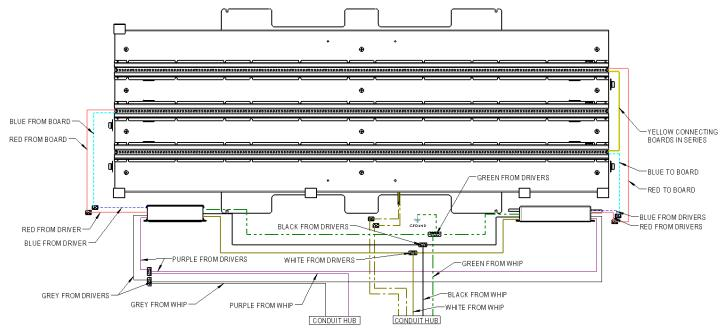
NOTE: DIMMING LEADS TO COME OUT OF LEFT CONDUIT HUB ALL OTHER LEADS TO COME OUT OF RIGHT CONDUIT HUB
