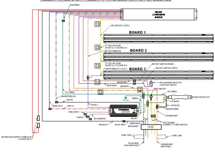
"D1" (0-10V Dim) option shown - Dimming Leads run out separate conduit hub.
